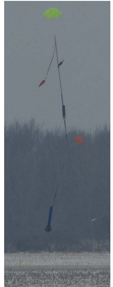
K.O.C.B. by Bert Wise powered by an Aerotech J 420 Redline. Great lift off, clean flight, perfect dual-deployment recovery.
